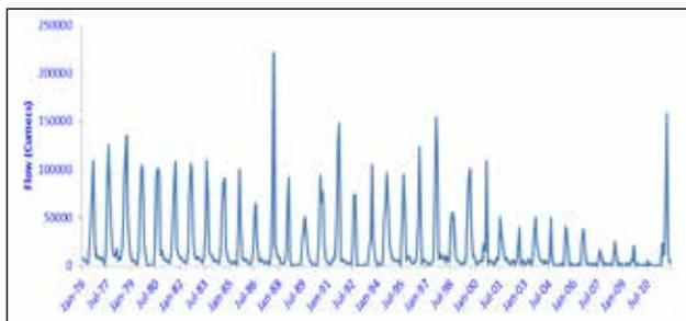
Fig. 9. Monthly water discharge from Indrapuri barrage (1976- 2011)
